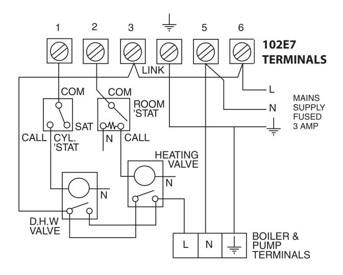
The above control system is available as the Danfoss Randall 102E7 HEATPLAN pack, which also includes the RMT room thermostat, AT cylinder thermostat, two 22mm HPP zone valves and a WB12 wiring box.
