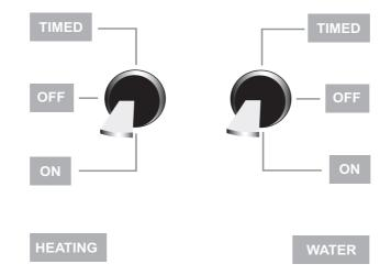
Each of the selector switches can be put into one of three positions marked 'TIMED', 'OFF' and 'ON'. They operate completely independently of one another, letting you select different programmes for each service.
