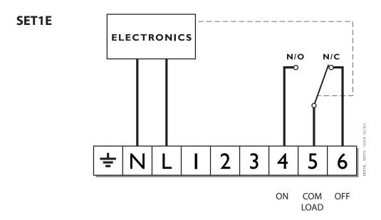
**NOTE:** For mains voltage applications a link must be fitted between terminals L and 5.
