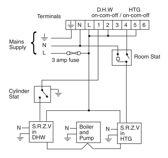
Other Danfoss Randall products suitable for use with above circuit:-AT cylinder thermostat;
