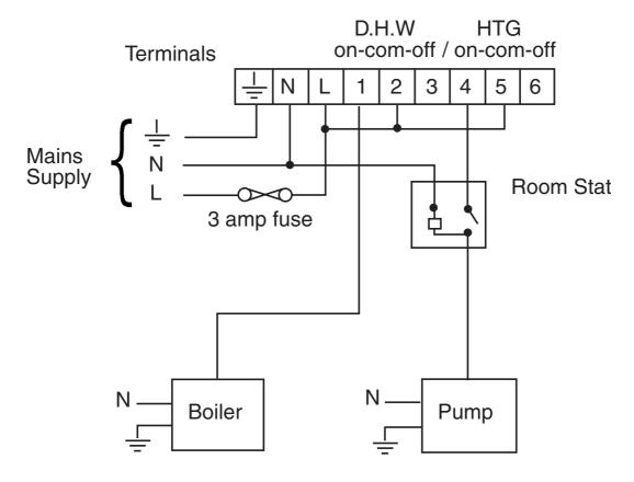
Other Danfoss Randall products suitable for use with above circuit:-RMT room thermostat
