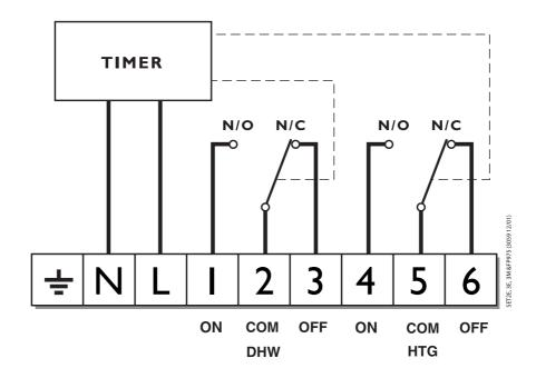
For mains voltage applications a link must be fitted between terminals L, 2 and 5.
