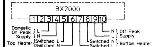
Wiring diagram for Hot water cylinders with dual or twin immersion heater.
