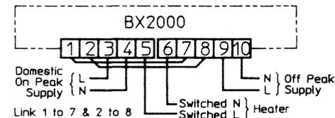
Wiring diagram for Hot water cylinders with single immersion heater.
