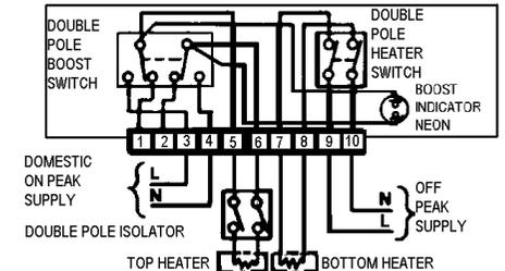
Wiring diagram for Hot water cylinders with dual or twin immersion heater.
